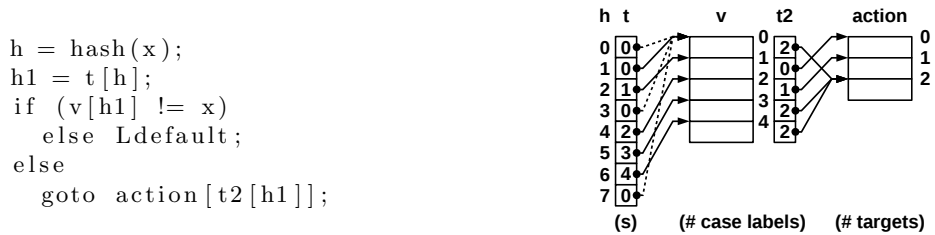
Fig. 5.3. C source for index mapping to compress hash range and jump tables
